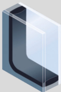
Structure with TPS ® applied by extrusion
