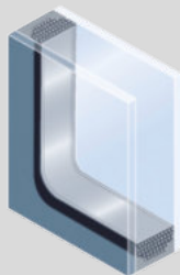
Traditional type of structure with metal profiles and drying salts
